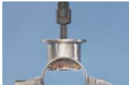
Sand and deburr inside small dia. pipe and other hard to reach areas with 3/4" - 1-1/2" stars.
