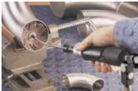
3" Eyelet Sanding Star easily enters pipe elbow using 7" long flexible mandrel.
